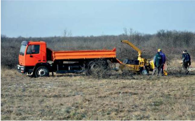
**Fig. 7.** The eradication of invasive woody species results in woody plant parts. A woodchipper is often used for reducing these parts into smaller woodchips. (Photo: M. Korda)
